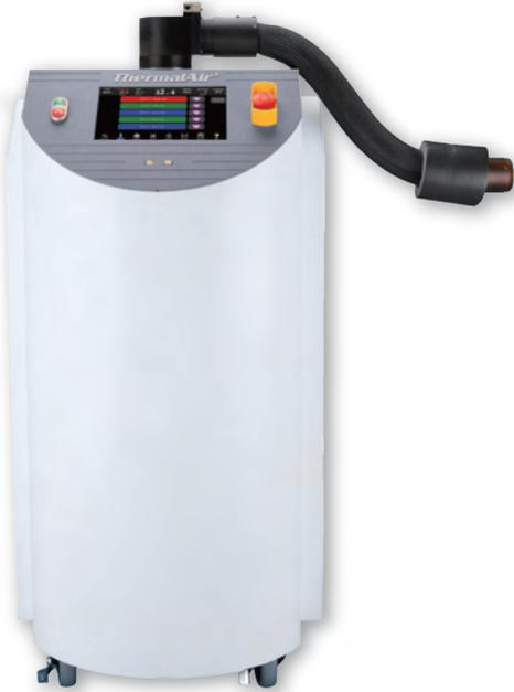
The ThermalAir TA-5000B high capacity thermal air stream system is used for temperature testing, fast thermal cycling, and device temperature characterization of components, hybrids, modules, PCBs, and other electronic and non-electronic assemblies at precise temperatures from  $-80^{\circ}\text{C}$  to  $+225^{\circ}\text{C}$ .
